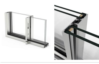
Avant-garde Sliding system design with thermal break which seeks maximum luminosity with minimum aluminium profile division view of market, just 2cm. and allows the possibility of closing large gaps up to 13.2 (width) x 3 ( height) meters in 6 sashes.
